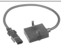
EAC sensors typically have a thin temperature probe that is glued inside a hole between the coolant tubes in the radiator. This plastic probe breaks off if the sensor is removed, which prevents the sensor from being swapped to a non-DOR radiator.
